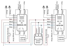
By using two low-voltage switches, a ceiling sensor and two BZ-150s (one set to Auto ON and one set to Manual ON) bi-level switching with manual-on operation can be achieved.
